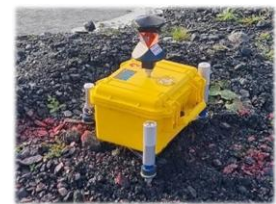
GAIA-FIELD with total station for <1 cm vertical accuracy during \mu Gal survey
